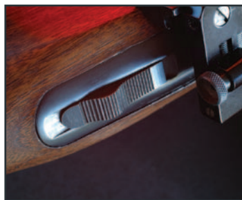
TOP: F.H. Rigall harvested this Alberta sheep in 1906 with his Savage 99. LEFT: When protruding, this peg shows a Savage Model 99 is cocked. It debuted on the Model 1899. ABOVE: This 1971 Model 99-A has the two-position tang safety standard on all post-1961 Savage 99s.
