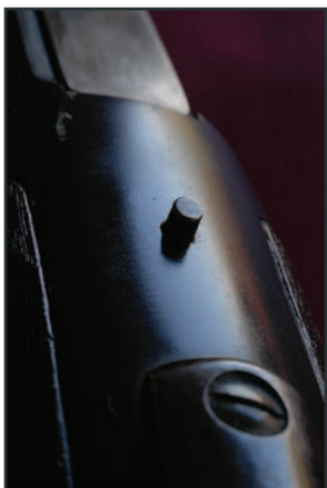
TOP: F.H. Rigall harvested this Alberta sheep in 1906 with his Savage 99. LEFT: When protruding, this peg shows a Savage Model 99 is cocked. It debuted on the Model 1899. ABOVE: This 1971 Model 99-A has the two-position tang safety standard on all post-1961 Savage 99s.
