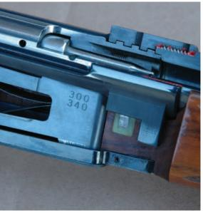
TOP: This cutaway shows the Mark V's interrupted-thread lockup, its full-diameter bolt, glass bedding in the recoil lug abutment. The magazine box is for the full-length .300 and .340 Magnums.
